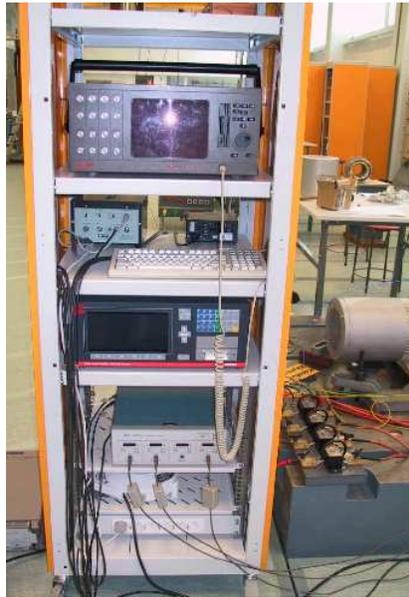
*Fig. 4.7 Measurement devices. From top to bottom: transient recorder, keyboard, power analyser, isolation amplifier, and connection box.*
