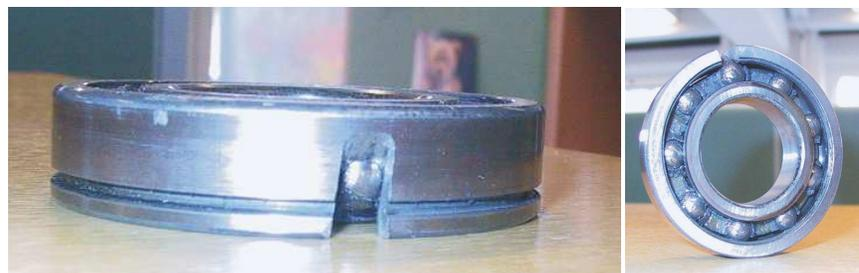
*Fig. 2.5 Artificially created bearing fault studied in this work.*
