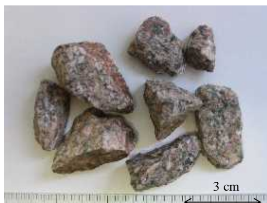
Figure 17 Rock used as abrasive material in the tests is slightly red granite.
