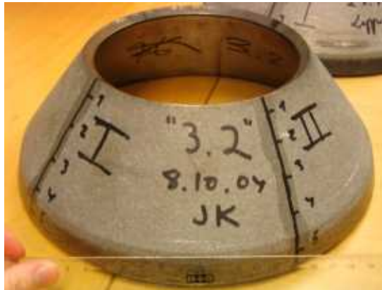
Figure 18 Laboratory cone crusher wear part, mantle and measuring stick of 20 cm are shown in the picture.
