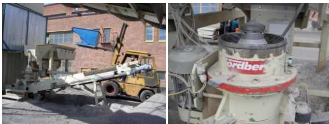
a) b) Figure 16 a) The forklift truck is filling the feeder of B90 cone crusher, b) open B90 equipment, and the upper part of the mantle is seen in the figure.
