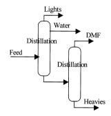
Fig. 8. The train with a combined operation.
