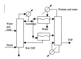
Fig. 6. Separation strategy found for azeotropic distillation with phase split.
