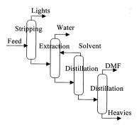
Fig. 9. The train with extraction separation.
