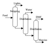
Fig. 7. Train of single distillation separations.
