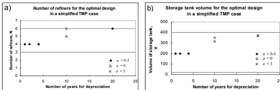
Figure 2. Risk premium weighing effect ( $a = 0 - 3$ ) on the optimal design in the simplified TMP case with different number of years for depreciation: (a) number of refiners and (b) storage tank volume.
