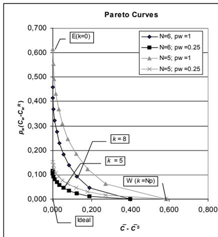
Figure 3. Robust optimization of the simplified TMP case with four different demand scenarios of the paper machine. The best robust solutions based on the worst-case analyses are found with  $N = 6$  and with the indexes  $k = 5$  and  $k = 8$  for the different scaling factors (probability of the worst-case scenario)  $p_w = 0.25$  or  $p_w = 1$  (no scaling), respectively. The optimum solution with  $p_w = 0.25$  corresponds the storage tank volume of  $V_{\text{tank}} = 350$ .
