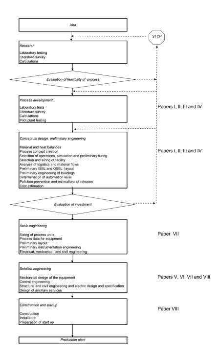
Figure 1. Process design stages (based on Aittomäki et al. 2002). Steps where the methods presented in Papers I to VIII can be applied are also pointed out.
