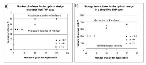
Figure 8. Risk premium weighting effect (a = 0 to 3) on the optimal design in the simplified TMP case with different number of years for depreciation: (a) number of refiners and (b) storage tank volume.
