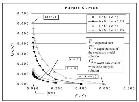
Figure 9. Robust optimization of the simplified TMP case with four different demand scenarios of the paper machine. The best robust solutions based on the worst case analyses are found with N = 6 and with the indices k = 5 and k = 8 for the different scaling factors (probability of the worst case scenario)  $p_w = 0.25$  or  $p_w = 1$  (no scaling), respectively.
