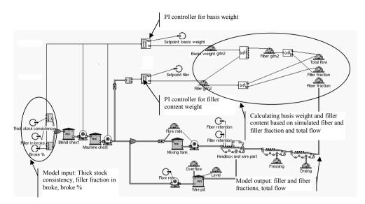
Figure 10. Simulation model with two PI controllers. The control loops are one for filler content and one for basis weight.
