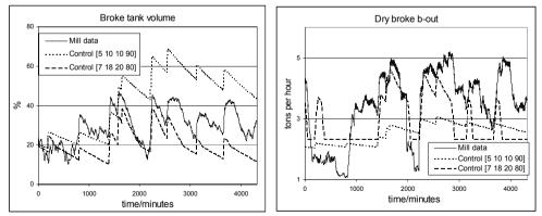
Figure 13. Broke tank volume and broke flow to paper machine, simulated and mill data
