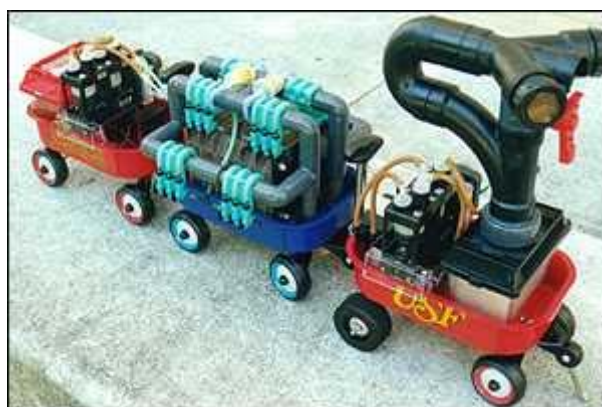
Figure 2.15. The gastrobot ( Chew-Chew ) runs on sugar cubes. (Courtesy of Stuart Wilkinson)
