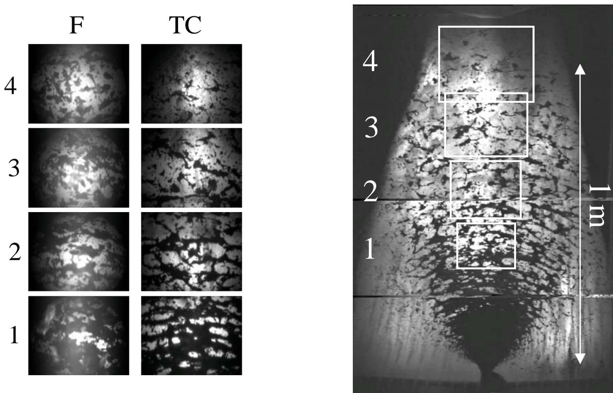
**Figure 3. Black liquor sheet break-up in the furnace (F) and in the test chamber (TC) at distances of 0.4 m (1), 0.6 m (2), 0.8 m (3) and 1.0 m (4) from the exit of the nozzle and the over-all view of the black liquor spray in the test chamber, nozzle A.**
