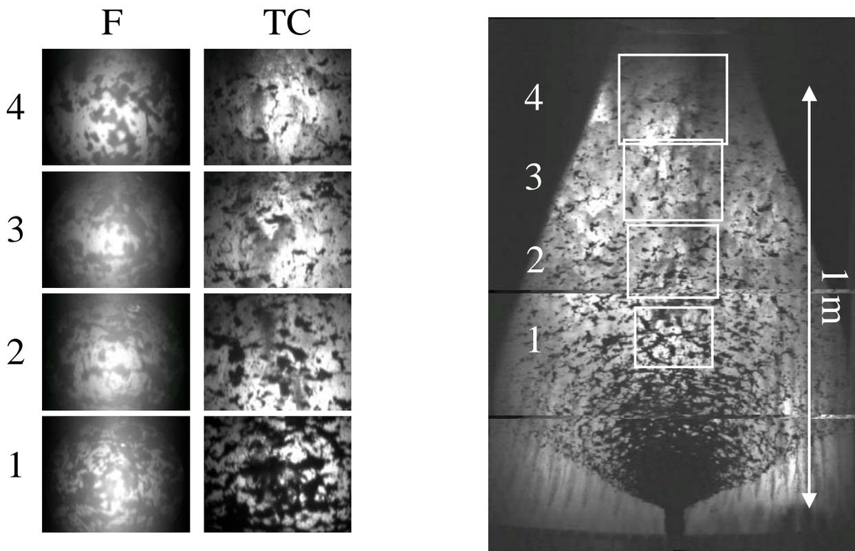
**Figure 4. Black liquor sheet break-up in the furnace (F) and in the test chamber (TC) at distances of 0.4 m (1), 0.6 m (2), 0.8 m (3) and 1.0 m (4) from the exit of the nozzle and the over-all view of the black liquor spray in the test chamber, nozzle B**
