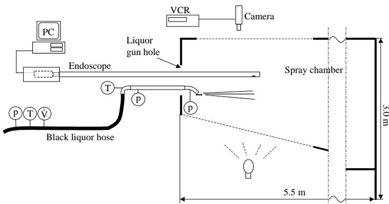
**Figure 2. Experimental configuration**
