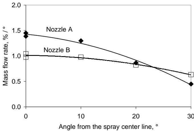
Figure 5. Distribution of the mass flow of nozzles A and B, 60 cm from the nozzle exit at a flow rate of 5.2 kg/s
