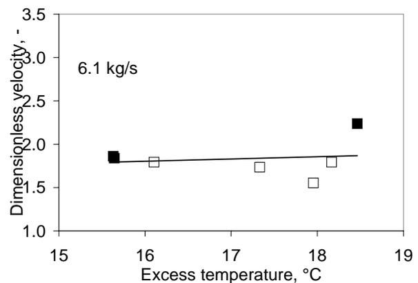
**Figure 6. Dimensionless velocity as a function of the excess temperature for nozzle A. The black diamonds represent the furnace and the open diamonds the test chamber.**
