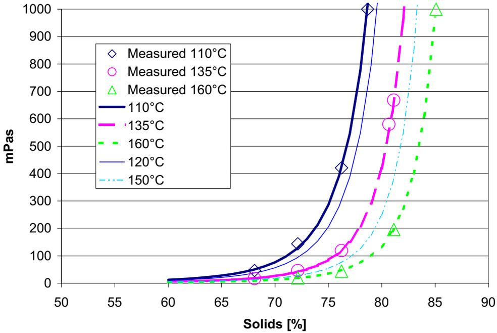
Figure A-1: Viscosity of high solids content black liquor at varying temperatures.
