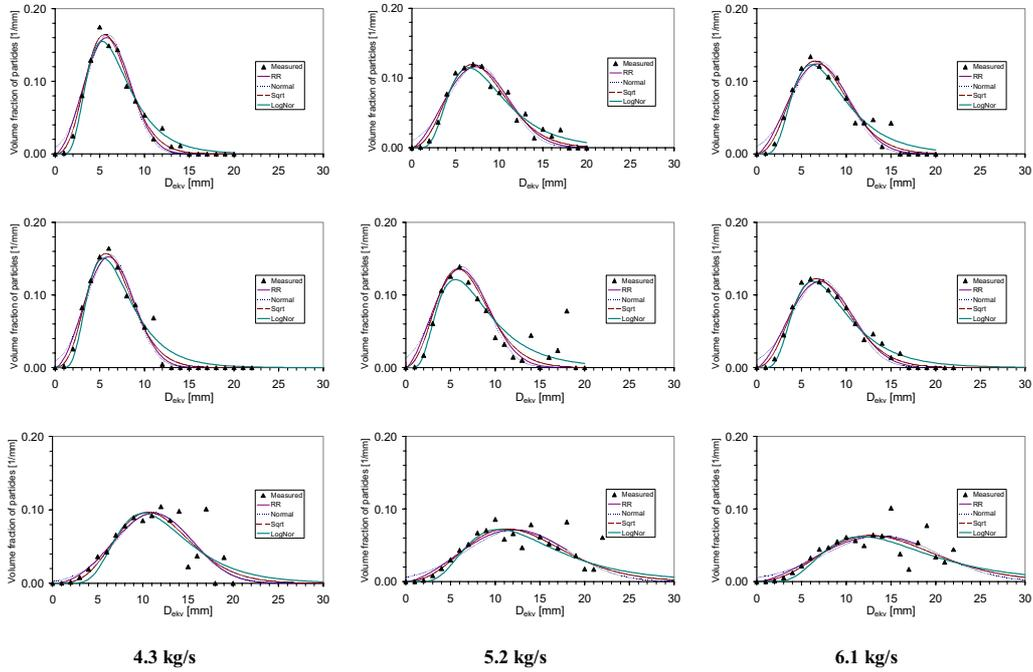
Figure 6: Particle size distribution of Nozzle A with fitted size distribution curves for nine spraying experiments, at excess temperatures of 14°C, 17°C, and 18°C in an upwards direction.
