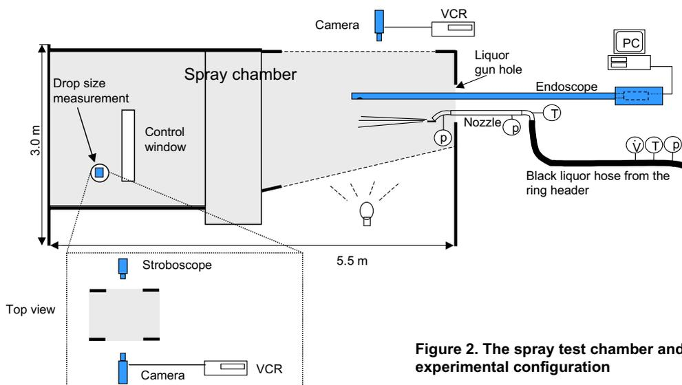
**Figure 2. The spray test chamber and experimental configuration**
