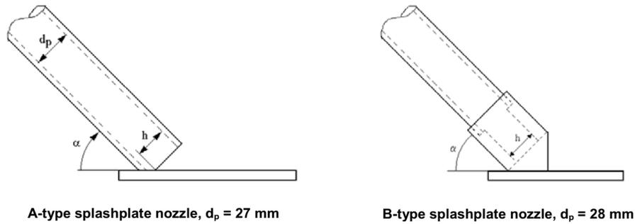
**Figure 1: Splashplate nozzles of types A and B**
