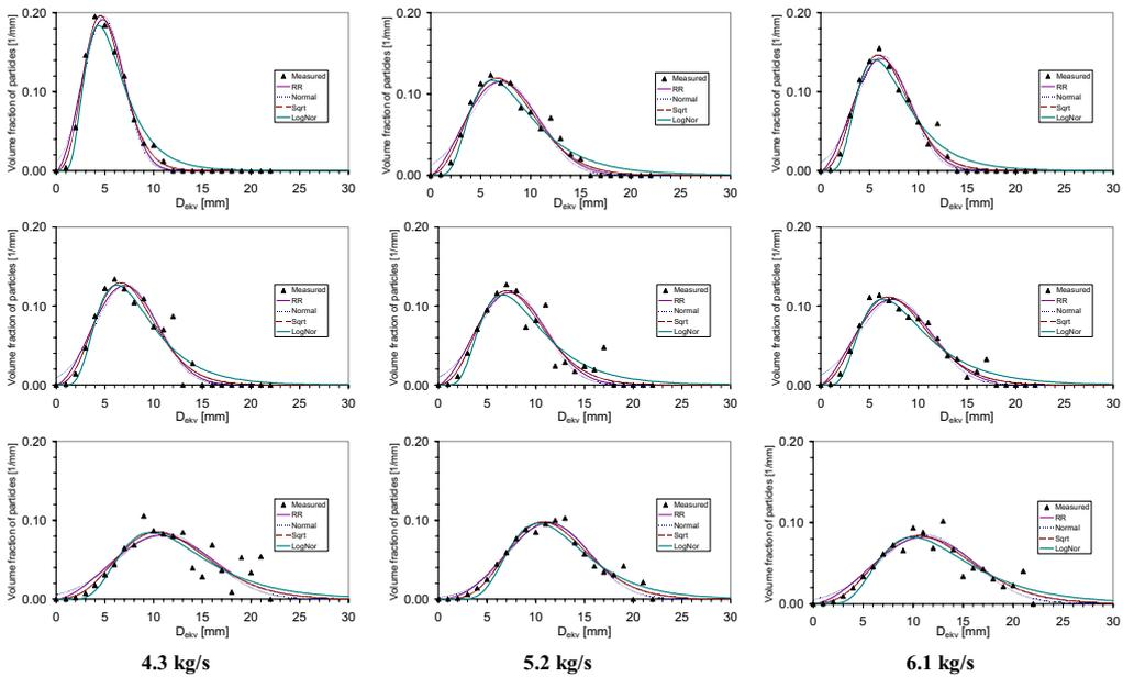
Figure 7: Particle size distribution of Nozzle B with fitted size distribution curves for nine spraying experiments, at excess temperatures of 14°C, 17°C, and 18°C in an upwards direction.
