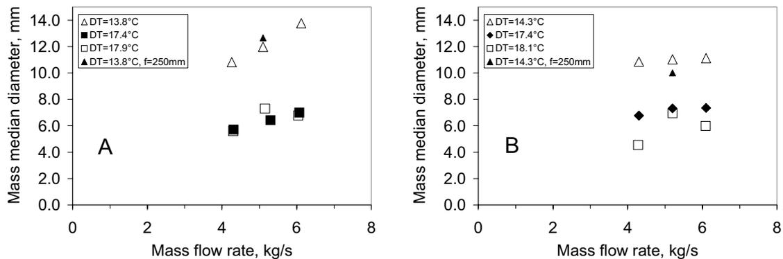
Figure 5. The effect of mass flow rate on combined median drop size, Nozzles A and B
