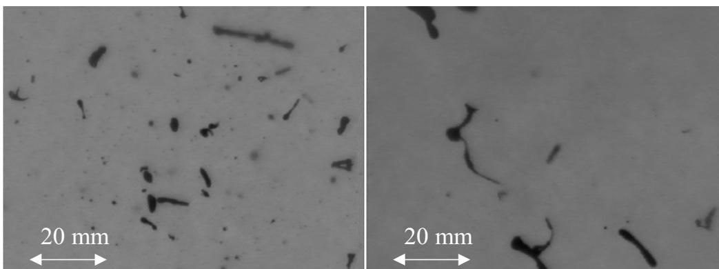
**Figure 3. Particles in two spraying situations at a distance of 4 meters from the nozzle. High solids content black liquor 4.2 kg/s at a spraying temperature of 135°C (left) and 6.1 kg/s at a spraying temperature of 130.4°C (right).**
