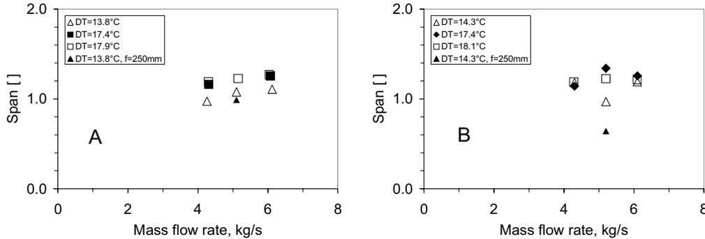
**Figure 8: The effect of mass flow rate on the span of experimental drop size distribution for Nozzles A and B**
