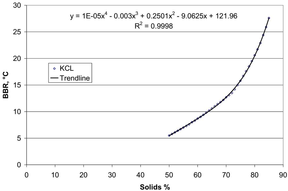
Figure A-2: The boiling point rise of high solids content in black liquor.
