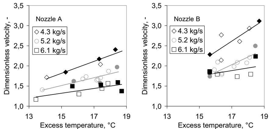
Figure 4. The effect of temperature on spray velocity
