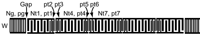
Fig. 1. Schematic of the test filter structure. The filter has 5 main transducers with short transducer sections replacing the gaps between them. The structure is symmetric such that it has 14 simultaneously optimized parameters as indicated in the figure.
