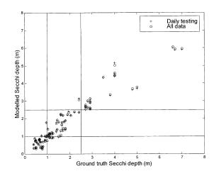
Fig. 4. Regression model for Secchi depth with AISA data. Vertical and horizontal lines represent quality class limits. Number of data points = 102. For all data,  $R^2 = 92.6\%$ ; for daily testing (separate training and testing data sets),  $R^2 = 91.8\%$ .
