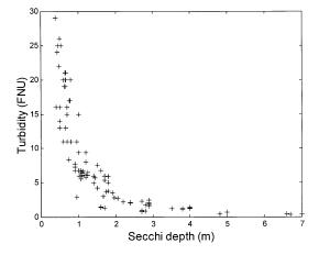
Fig. 1. The relationship between Secchi depth and turbidity.
