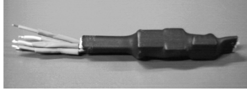
Fig. 1. A prototype with three sensors mounted together. Only two sensors are used in the current system.
