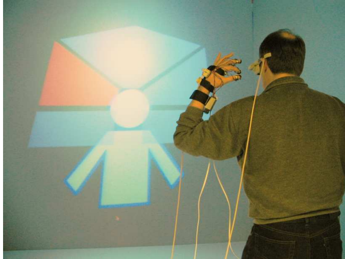
Figure 5.14: Visual area display in an otherwise empty world. The first pocket is on top of the left shoulder and fifth on top of the right shoulder (for right-handed users).
