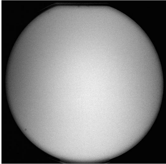
Figure 23. IR image of the same wafer as in Figure 22. 30 nm high patterns are too small to be detected by IR transmission.
