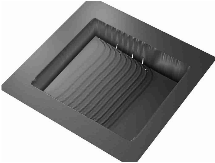
Figure 13. Optical profilometry image of an etched cavity on a Si wafer.
