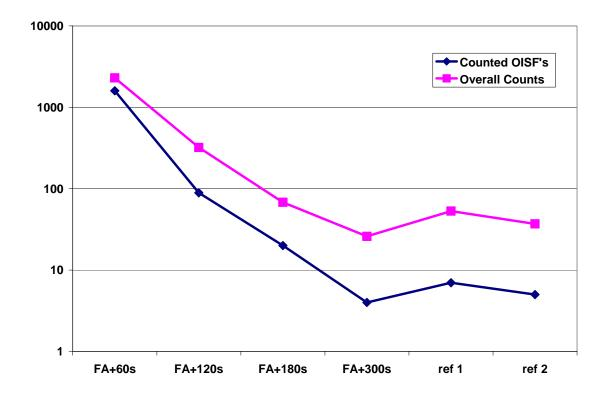
**Figure 3**: OISF counts on a diameter scan after different final polishing times. The count decreases rapidly with increasing the final polishing time and reaches reference level after 300s referring to 0.5 µm removal.
