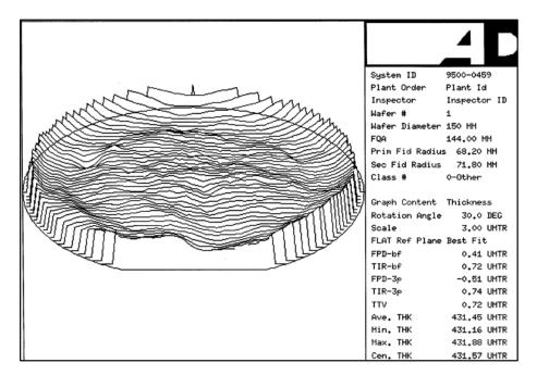
**Figure 2**: After final polishing and further 0.5 µm removal the wafer is still very flat. The last polishing step does not strongly influence the result.
