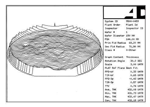
**Figure 1**: Capacitive thickness scan of the FA polished wafer. No edge rounding is visible. The overall TTV is well below 1 μm
