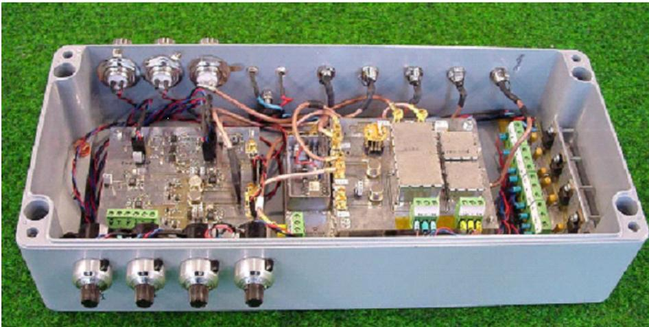
*Figure 41. Photograph of the DC voltage reference.*
