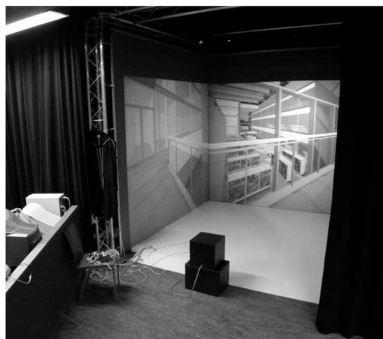
Figure 1: The virtual room of the Helsinki University of Technology. Loudspeakers are behind the screens. No visual stimulus was shown in experiments.
