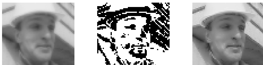
Figure 2.21 The low-pass filtered image, resulting mask and masked image using the resistive network only.
