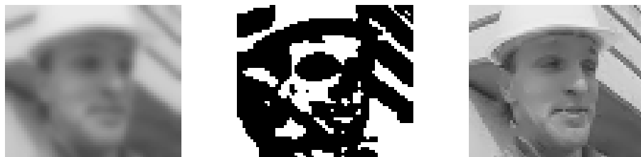
Figure 2.20 The low-pass filtered image, resulting mask and masked image using the method proposed in [14].
