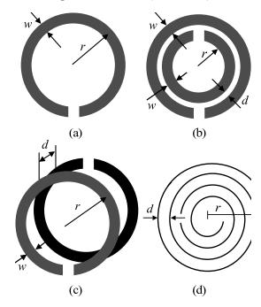
**Figure 1.** (a) Single split-ring resonator. (b) Split-ring resonator (SRR). (c) Modified split-ring resonator (MSRR) (d) Cross section of the Swiss roll.
