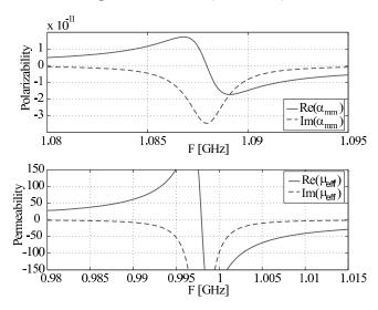
**Figure 6.** The polarizability  $\alpha_{\rm mm}$  (top) and the permeability  $\mu_{\rm eff}$  (bottom): analytical model.
