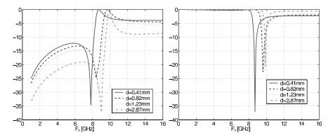
**Figure 10.** Results of HFSS simulations for the case of separate MSRR forming an artificial crystal. The  $S_{11}$  magnitude plot is given on the left and the  $S_{21}$  magnitude is on the right. The several curves on each plot correspond to different distances between the MSSRs in stacks (parameter d).
