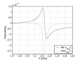
Figure 13. The real and imaginary parts of the metasolenoid polarizability  $\alpha_{mm}$  as functions of frequency: the measured results.
