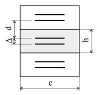
**Figure 9.** Definition of the simulation box for arrays of separate MSSR. As for the metasolenoid (Figure 7), the box containing only one pair of rings is bounded by magnetic walls on the top and bottom and by electric walls on the two sides. The rings are seen as bold lines (side view).
