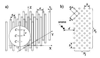
FIG. 1. (a) Geometry of capacitively loaded wire medium (CLWM). (b) Geometry of the crystal sample.
