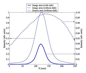
FIG. 7. (Color online) Measured intensity distribution along the axis x (parallel to the slab interface). The arrow indicates the scale which is used to read the intensity values. Intensity in the channeled field area has been measured at 10 mm distance from the slab interface. Intensity in the source area has been measured at 10 mm distance from the source.
