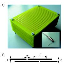
FIG. 3. (Color online) (a) The implemented CLWM crystal sample and the probe used in the measurements. (b) A schematic illustration of the loaded wire (a piece of it).
