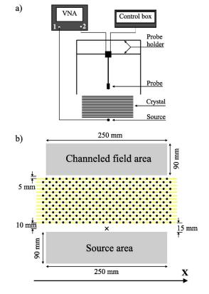
FIG. 4. (Color online) (a) A schematic illustration of the measurement setup. (b) The measurement area. The black dots denote the loaded strips, the cross denotes the source.
