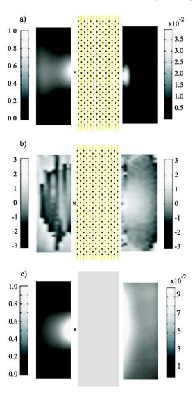
FIG. 6. (Color online) (a) The measured intensity distribution (in arb. units). (b) The measured phase distribution of electric field (in radians). (c) The measured intensity distribution without the CLWM crystal (in arb. units). In (a) and (c) the intensity values in the channeled field area have not been normalized to better see the details of the intensity distribution.
