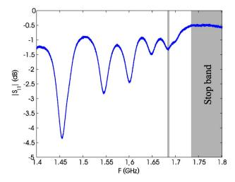
FIG. 5. (Color online) Measured  $S_{11}$ -level of the slab. The desired Fabry-Pérot resonance is shown with a vertical line.
