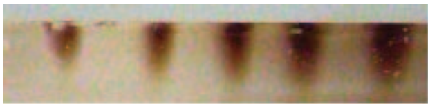
Fig. 3. Coloration caused by the UV exposure. Sample cross sections showing irradiated areas for different exposure times (from left to right): 0.9, 1.8, 3.6, 9, and 18 kJ/cm 2 .
