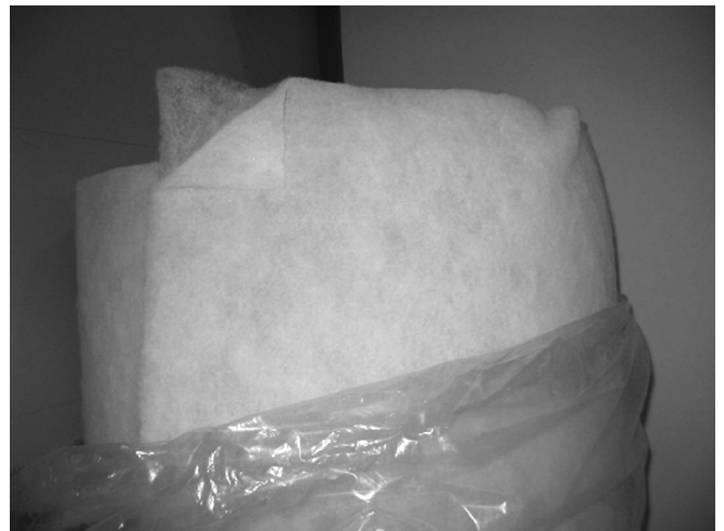
Figure 6 — Filter fabric, G3.
