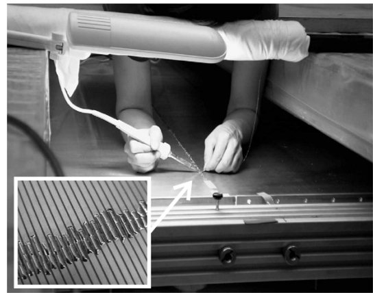
Fig. 6. Soldering of the 3-m-hologram. Soldered metal strips are shown in the inset.
