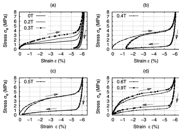
Fig. 1. Stress-strain curves for different values of the applied magnetic field. (a) For zero or small field, the sample is superplastic. (b) For a few cycles in the field of 0.4 T, the process is partly reversible. (c) Further increasing of field to 0.5 T brings more reversibility. (d) Strain is fully reversible for the field of 0.6 T and above.
