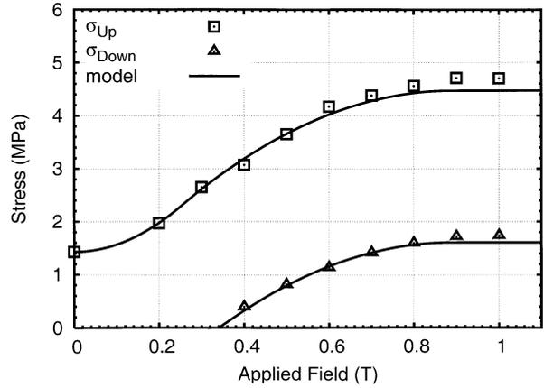
Fig. 5. External stress necessary to induce strain 3% ( $\sigma_{Up}$ , squares) and stress induced by magnetic field at strain 3% ( $\sigma_{Down}$ , triangles) during sample unloading as functions of the applied field. Solid line shows calculation from the model.
