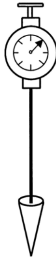
Figure 3.3 Cone penetrometer. The standard cone consists of a 30° circular cone with a half-square-inch base area equal to 322,6 mm 2 .
