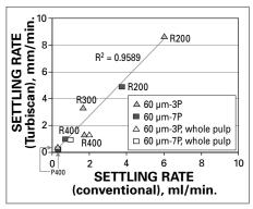
4. Settling rate of fines fractions measured with two different techniques.
