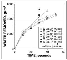
3. Dewatering rate of fines suspensions containing different amounts of fines.
