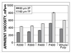
5. Apparent viscosity of fines fractions. Brookfield viscosity at 100 rpm with spindle No. 3.
