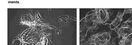
2. Microscopic images of fines (P100 fraction), 60 μm-7P. Phase contrast mode (left) and bright field with polarized light mode (right).
