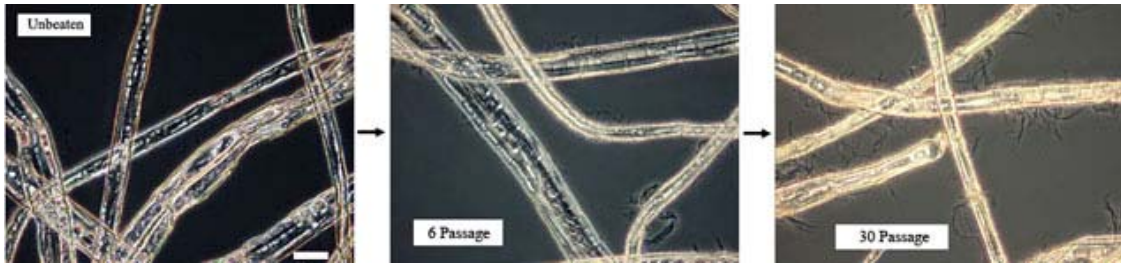
Fig. 5.4 Light microscopic observation of external fibrillation of fibers (R100 fraction). Once-dried bleached kraft softwood pulp with 5% consistency treated at the gap of 240 \mu\text{m} in the grinder. Scale bar of 50 \mu\text{m} . [V].
