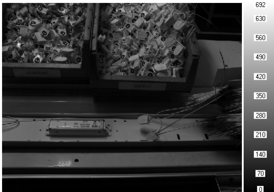
Figure 13. Luminance distribution of one assembly table in study C. ( \text{cd/m}^2 )
