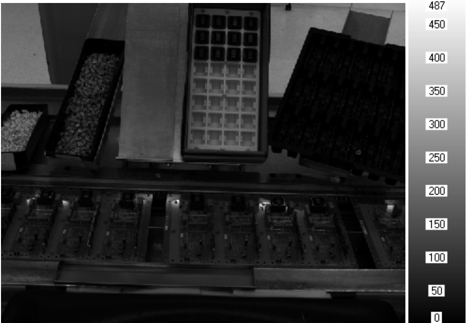
Figure 16. Example of the luminance distribution of workstation of study D (cd/m 2 )
