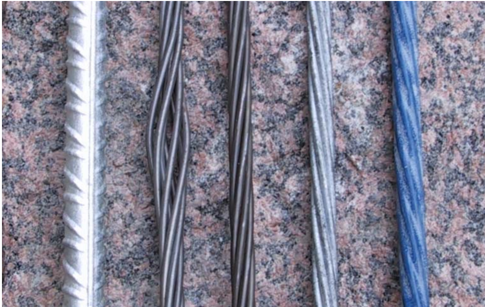
Figure 7. Test bolt types. From left: Rebar (with hot-dip galvanizing in the figure), bulbed strand, standard steel strand, hot-dip galvanized steel strand and epoxy-coated steel strand (Satola & Hakala 2001b).
