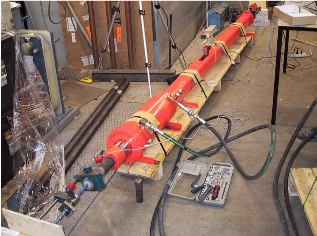
Figure 3. Double pipe axial testing machine (Satola & Hakala 2001a).
