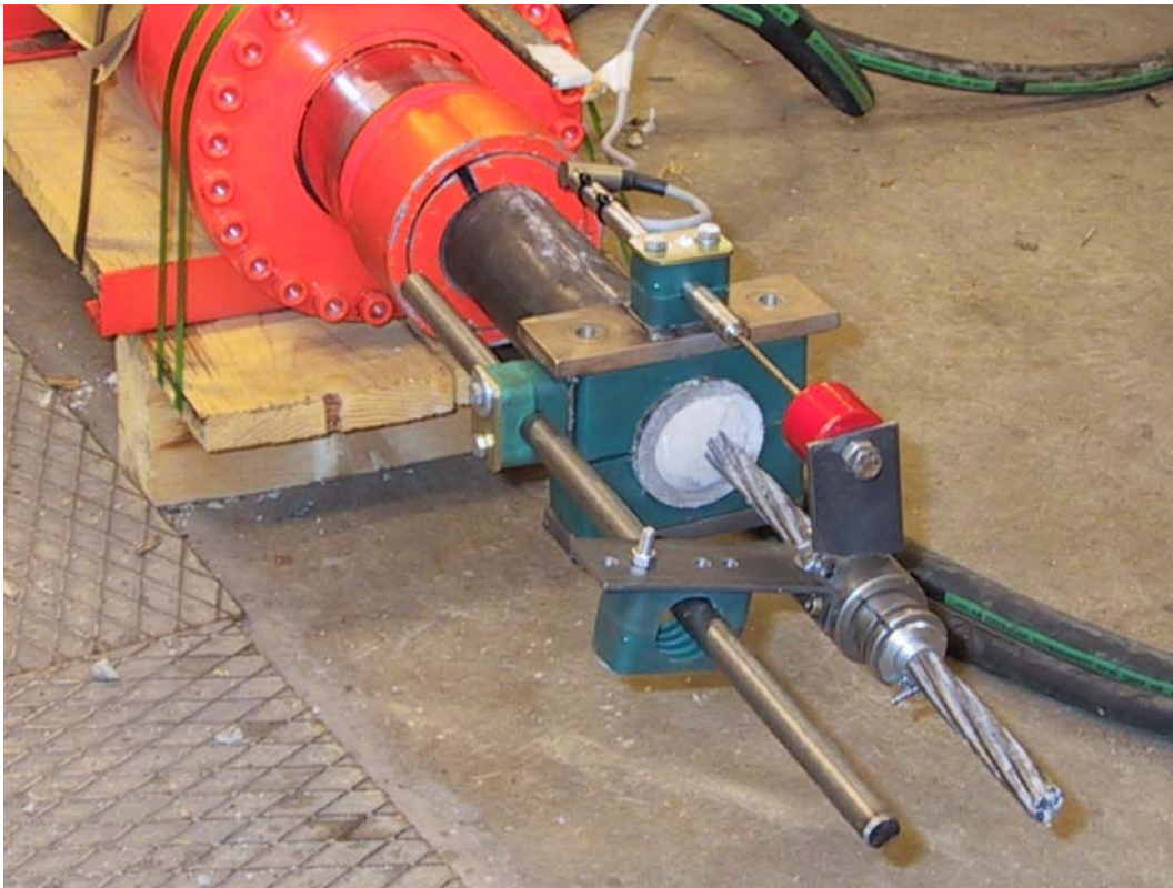
Figure 4. The connection of the displacement transducer to the test strand (Satola & Hakala 2001a).
