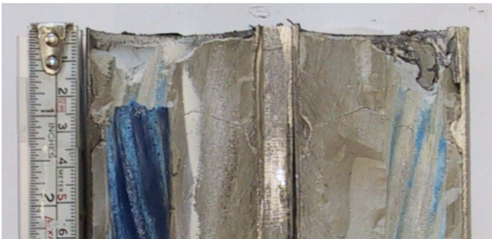
Figure 9. The split test pipe and the grout column after the test. Welded ring inside surface of the pipe (30 mm from the end of the pipe in the figure).
