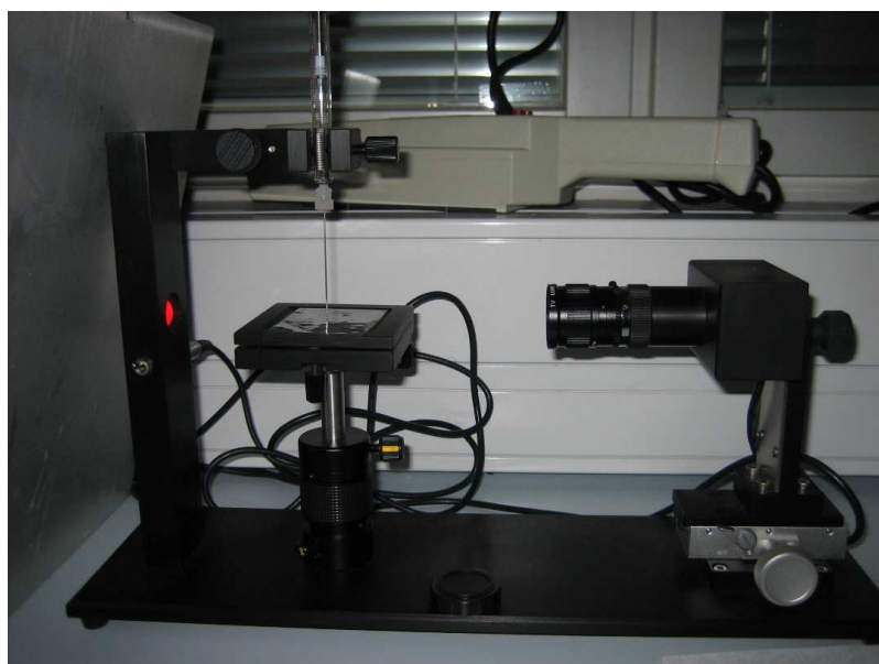
Figure 5.1: The goniometer used in water contact angle (CA) measurements.
