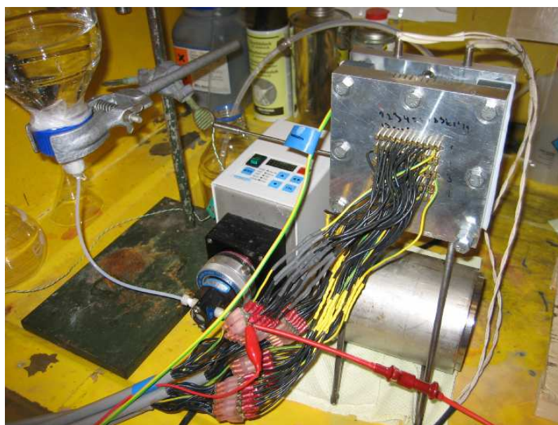
Figure 5.4: The free-breathing DMFC and the measurement system for the cathode current distribution.
