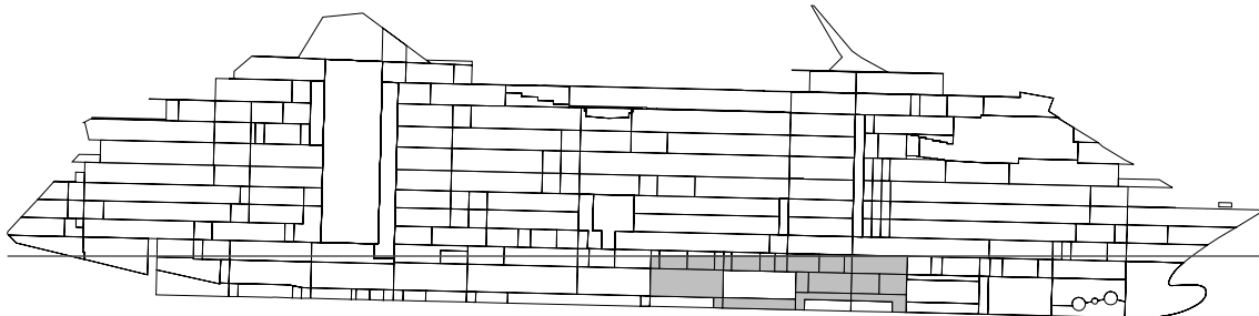
Figure 6.15 Floating position in the final equilibrium condition (the white parts in the four damaged compartments are the non-flooded tanks)
