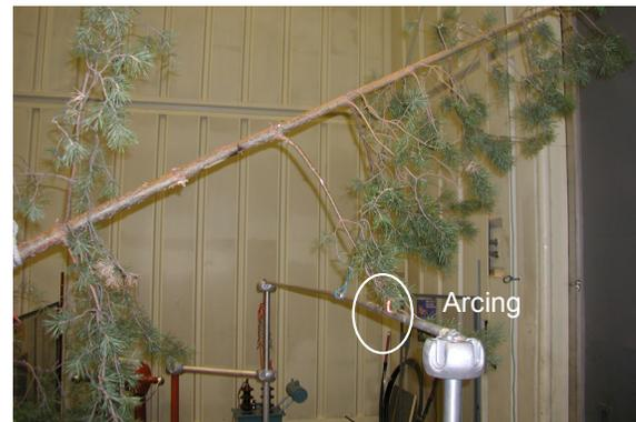
Figure 2. Arc-associated tree bending over the conductor.
