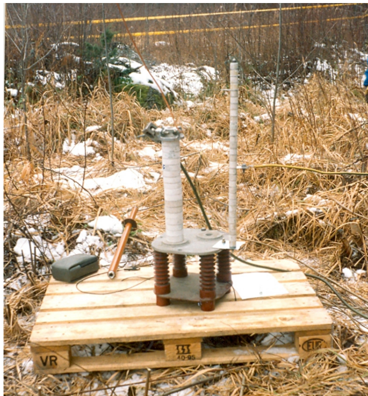
Figure 5.8 The resistance used as a fault object.
