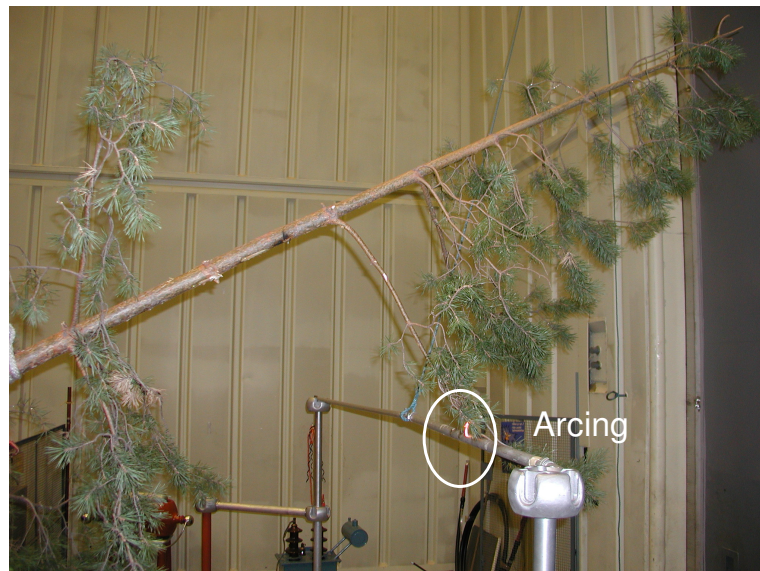
Figure 3.2 Arc-associated tree bending over the conductor.
