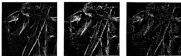
Fig. 9. Total ion image (left) and distribution of lignin (middle) and extractives (right) on the surface of TMP bulk fibers. The images were obtained by positive ion TOF-SIMS imaging. Scale: 100 \mu\text{m} .
