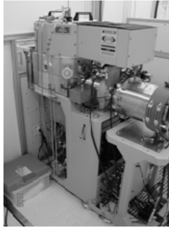
Fig. 3. Photograph of ICP etcher used in Si etching. (Picture courtesy of Gao Feng.)
