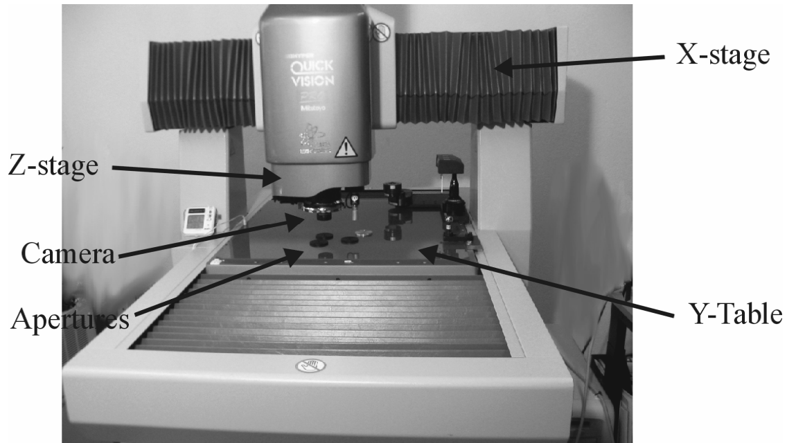
Figure 9. The optical CMM at MIKES.
