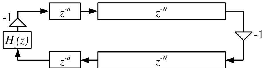
**Figure 3.1:** A simple DWG string implementation consists of two delay lines, a fractional delay filter for applying the fractional part of the delay, and a loop filter for simulating losses (after [Smith, 1992]).
