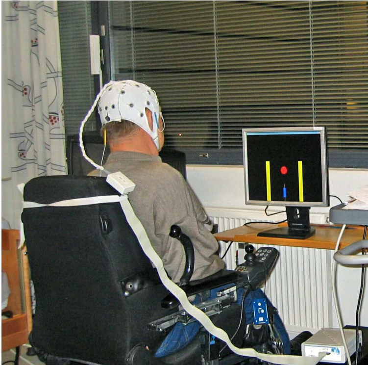
Figure 3.2: Subject sitting in front of the computer screen with EEG cap on. The subject's task is to move the red circle on the screen to the yellow target by attempting hand movements when the blue meter disappears.
