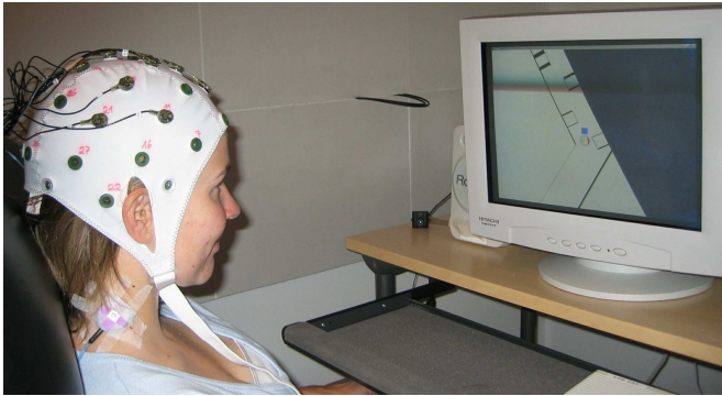
Figure 3.3: Subject sitting in front of the computer screen with the EEG cap on. She is trying to control the autonomous wheelchair robot by imagining hand movements. She received either visual feedback or vibrotactile feedback. The vibrotactile sensors are attached to the lower neck.
