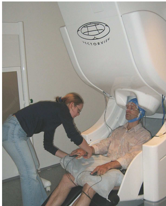
Figure 3.1: Subject is being prepared for simultaneous MEG and EEG measurement.
