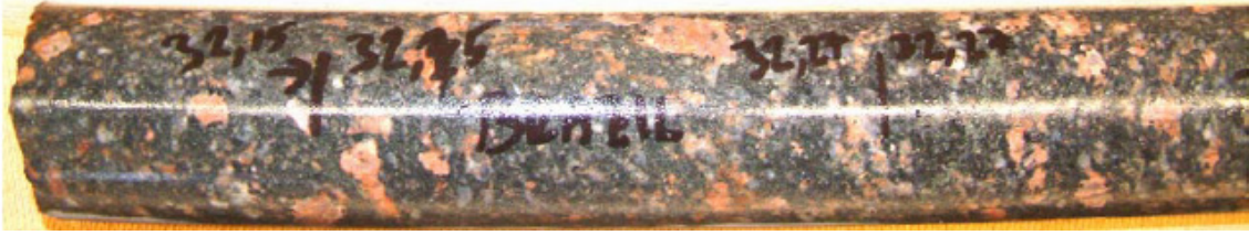
Figure 5-1. Typical unaltered Äspö diorite (Staub et al. 2004).
