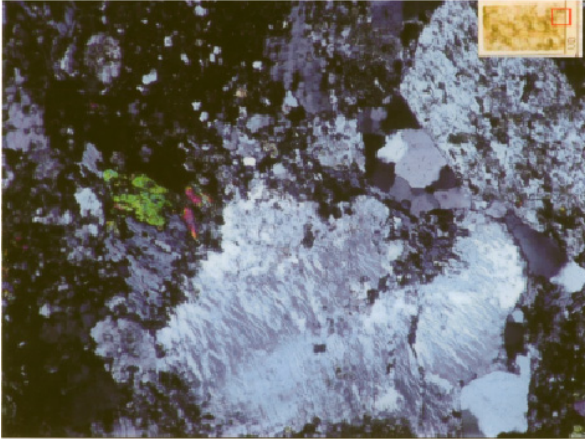
Figure 5-2. Unaltered Äspö diorite in polarised light. The feldspar grain has flame-like perthite lamellae. The width of the image is 4 mm (Lampinen 2006).
