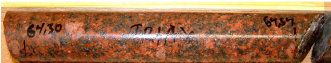
Figure 5-3. Oxidised Äspö diorite (Staub et al. 2004).
