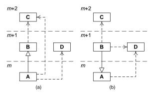
**Fig. 15** Generalisations between classes on different levels are not possible. (a) Subclass on a level below its superclass. (b) Subclass on a level above its superclass.
