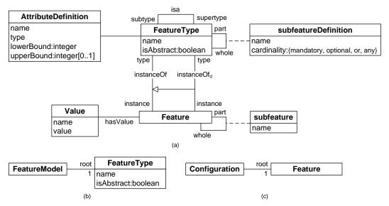
Fig. 12 The Forfamel metamodel as a UML class diagram. (a) Classes related to feature types and features, (b) feature model and (c) configuration. Adapted from [1]
