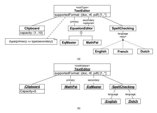
Fig. 14 (a) A sample feature model. (b) A sample feature configuration that is valid with respect to the above model.
