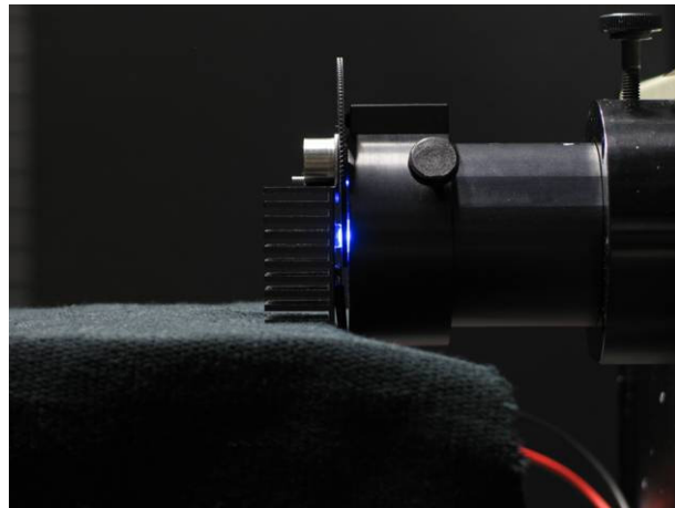
Figure 1- Measurement set-up used to determine the radiant intensity of the LEDs under known operational conditions using a monochromator-based spectroradiometer (754-C, Optronics Laboratories Inc., USA).
