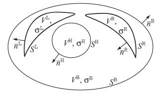
Figure 1: The piece-wise homogeneous model of the thoracic volume conductor;  $S^l$  labels the exterior boundary surface of the volume  $V^l$ , and  $\sigma^k$  is the conductivity in  $V^k$ . Superscripts mark the surfaces as follows: H is the epicardial (heart), L is the left lung, R is the the right lung, and B is the body surface. Normal vector  $\vec{n}^l$  points outwards from volume  $V^l$ .
