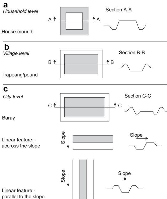
Fig. 3. Schematic illustration of the water management levels and typical associated structures. The different levels include: (a) household, (b) village, and (c) city levels (adapted from Pottier, 1999).
