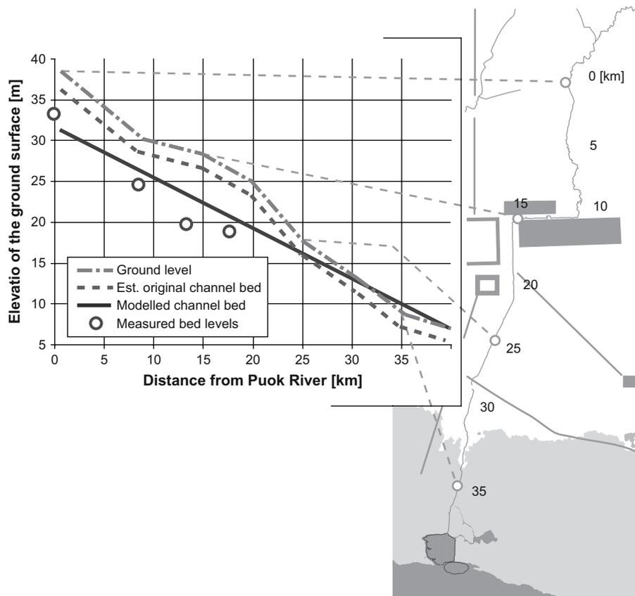
**Fig. 6.** The result of mathematical modelling of the down-cutting of the Siem Reap Channel. The dotted line is the original long section inferred for the bottom of the channel, while the solid one is the bottom of the channel after it stabilises (updated and modified from Lustig et al., 2008).
