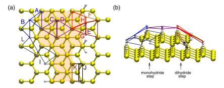
**Figure 1.** The most important adsorption sites on the H-terminated Si surface found at monohydride steps (A, B), (111) terraces (C, D), horizontal dihydride steps (E–H), vertical dihydride steps (J, K) and kinks (I, L). The large yellow (grey) spheres are Si and the small white ones are H. The surface is shown from (a) top-down and (b) side perspectives. Two layers of silicon are shown and the upper layer is shaded in (a) to show the steps better.
