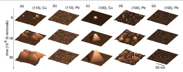
Figure 6. Evolution of the (110) ((a)-(b)) and (100) ((c)-(e)) surface morphologies in KMC simulated etching under the influence of Cu (clustering impurities) ((a) and (c)) and Pb (individually adsorbing impurities) ((b), (d), and (e)). In (e), the removal rates of monohydride step and kink sites are a factor of ten higher than in (d). The size of the simulated systems is  $120 \text{ nm} \times 120 \text{ nm}$ . Impurities are shown as white dots.
