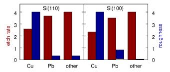
**Figure 7.** Average etch rate (left, red (grey) bars) and roughness (right, blue (black) bars) of simulated  $120 \text{ nm} \times 120 \text{ nm}$  (110) and (100) surfaces with Cu, Pb, and other impurities in arbitrary units. The (110) results are for high and (100) for low etchant concentrations. For Pb on (100), the blue (black) and white bars correspond to the morphologies in figures 6(d) and (e), respectively.
