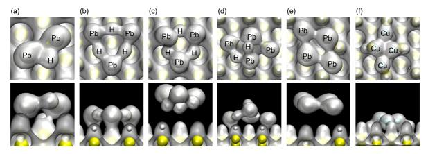
**Figure 4.** Electron densities of (a) a Pb<sub>2</sub>H dimer, (b) a Pb<sub>3</sub>H<sub>3</sub> trimer, (c) a Pb<sub>3</sub>H<sub>3</sub> trimer on a H-terminated surface, (d) a Pb<sub>4</sub>H<sub>2</sub> tetramer, (e) a Pb<sub>4</sub> tetramer, and (f) a Cu<sub>4</sub> tetramer shown from top-down and side perspectives. The densities are drawn at an isosurface of 0.014 e Å<sup>-3</sup> for Pb and 0.019 e Å<sup>-3</sup> for Cu.
