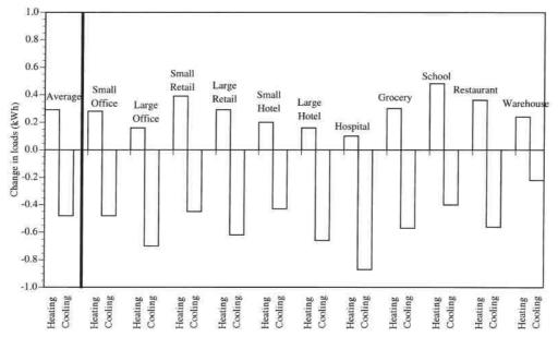
Figure 8 Changeinheatingandcoolingloadscausedbya1k commercialbuildings[Sezgan2000]
