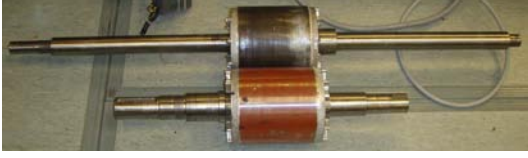
Fig. 6. The extended (length 1560 mm) rotor (above) used in the test machine and the standard rotor (below).
