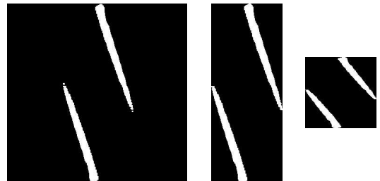
Fig. 2: Three normalization steps: 1) thresholding, 2) time gating and frequency filtering, and 3) aspect ratio normalization.
