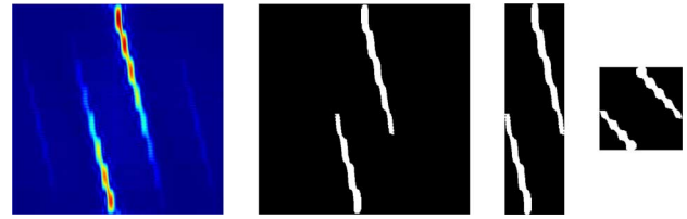
Fig. 6. The CWD normalization procedure starting from the original image (from left to right): 1) thresholding, 2) time gating and frequency filtering, and 3) aspect ratio normalization.
