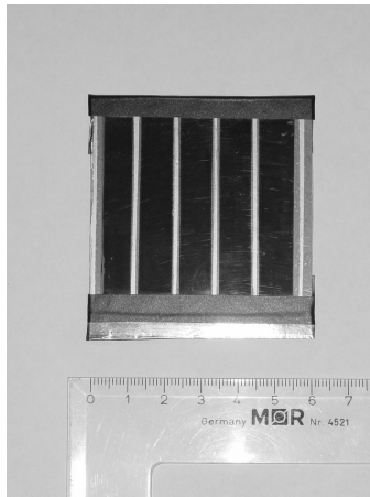
Figure 4.6 Example of a StS DSC with a larger active area.
