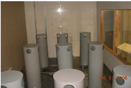
Figure 3.1 Photograph of the first test chamber with nine simplified cylindrical dummies.
