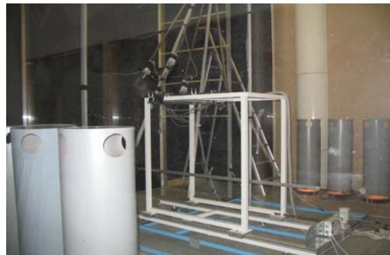
Figure 3.2 Photograph of the second test chamber with nine simplified cylindrical dummies.
