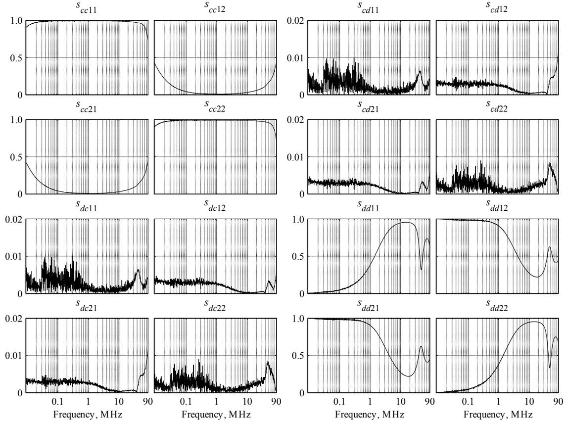
**Figure 5:** Mixed-mode  $s$ -parameters obtained from the single-ended  $s$ -parameters in **Figure 4**
