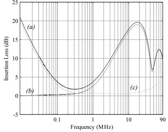
**Figure 7:** *a)*  $IL_{DM}$  measured in the symmetrical test circuit in Figure 1*b*, *b)*  $IL_{DM}$  calculated from the four-port network parameters, measured in the unsymmetrical test circuit in Figure 1*c*, *c)*  $IL$  of the baluns without filter
