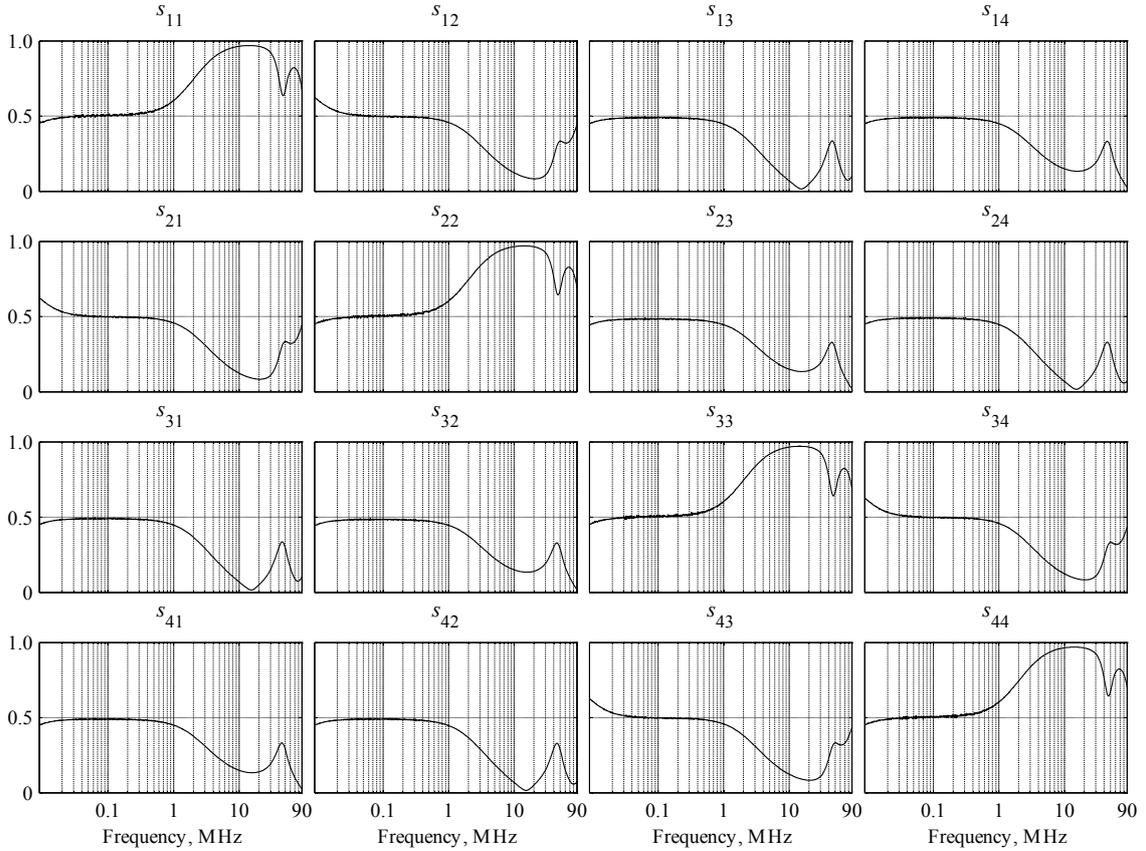
**Figure 4:** Measured single-ended  $s$ -parameters of the EUT
