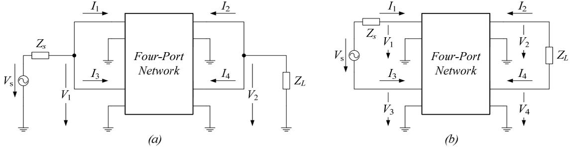
**Figure 3:** Set up for measuring  $IL$ : a) common-mode  $IL$ , b) differential-mode  $IL$
