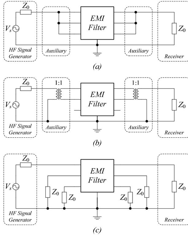
**Figure 1:** *IL* measurement test circuits:
