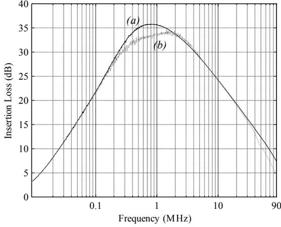
**Figure 6:** *a)*  $IL_{CM}$  measured in the asymmetrical test circuit in Figure 1*a*, *b)*  $IL_{CM}$  calculated from the four-port network parameters, measured in the unsymmetrical test circuit in Fig. 1*c*
